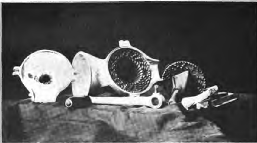
Figure 1—GRINDING SURFACES OF COAL CRUSHER.
